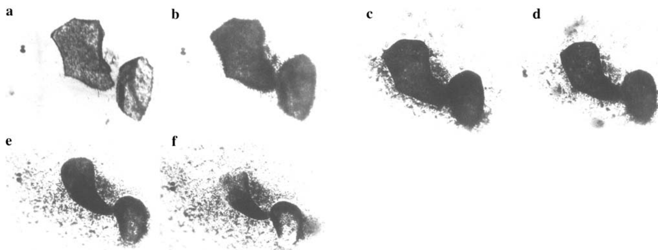
Fig. 3 Example of the dissolution of individual FAP crystals under conditions of \text{CaSO}_4 \cdot 0.5\text{H}_2\text{O} coating formation. Experimental conditions: 52% \text{H}_3\text{PO}_4 , 2% \text{H}_2\text{SO}_4 , t = 80^\circ\text{C} , Re \leq 100 , 75 \mu\text{m} \leq R_{\text{eq}} \leq 125 \mu\text{m} . Dissolution time: a – 15 s, b – 1 min, c – 45 min, d – 90 min, e – 128.5 min, f – 135 min. Magnification \times 90 . Horizontal field width = 1 mm
